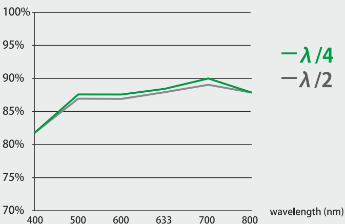
Typical transmission of laminated, uncoated mica waveplates (test result)
